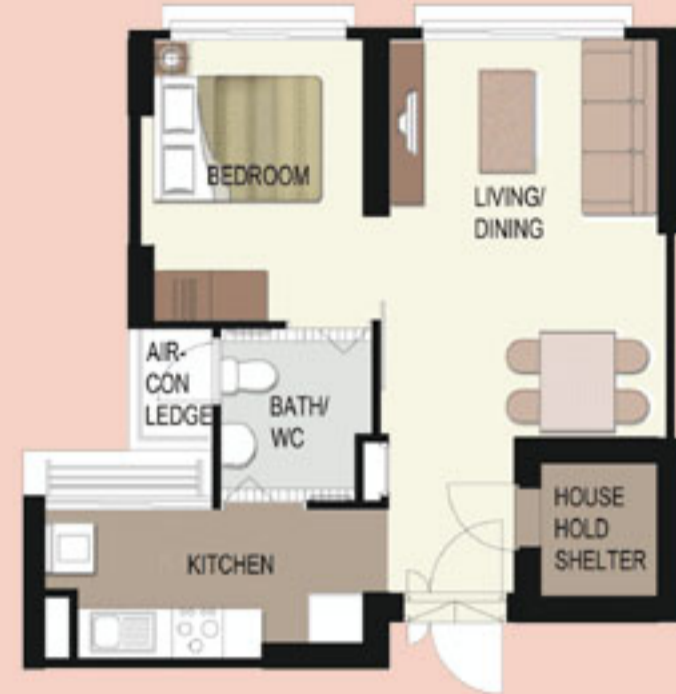
TYPICAL STUDIO APARTMENT (TYPE B) FLOOR PLAN APPROX. FLOOR AREA 47 sqm (Inclusive of Internal Floor Area 45 sqm and Air-Con Ledge)
