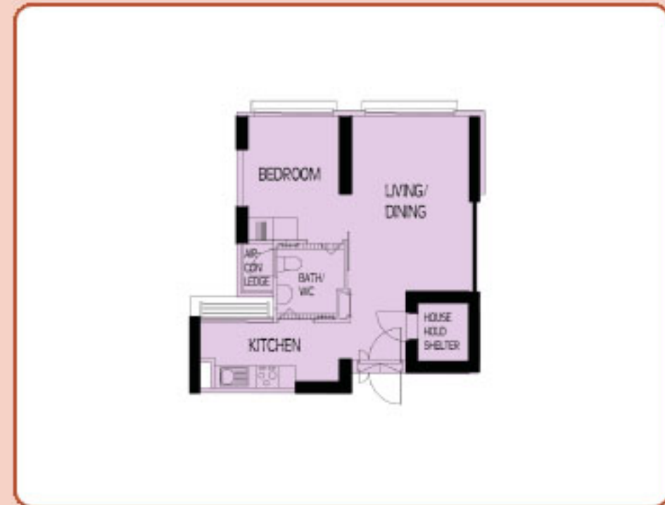
TYPICAL STUDIO APARTMENT (TYPE B) FLOOR PLAN APPROX. FLOOR AREA 47 sqm (Inclusive of Internal Floor Area 45 sqm and Air-Con Ledge)
