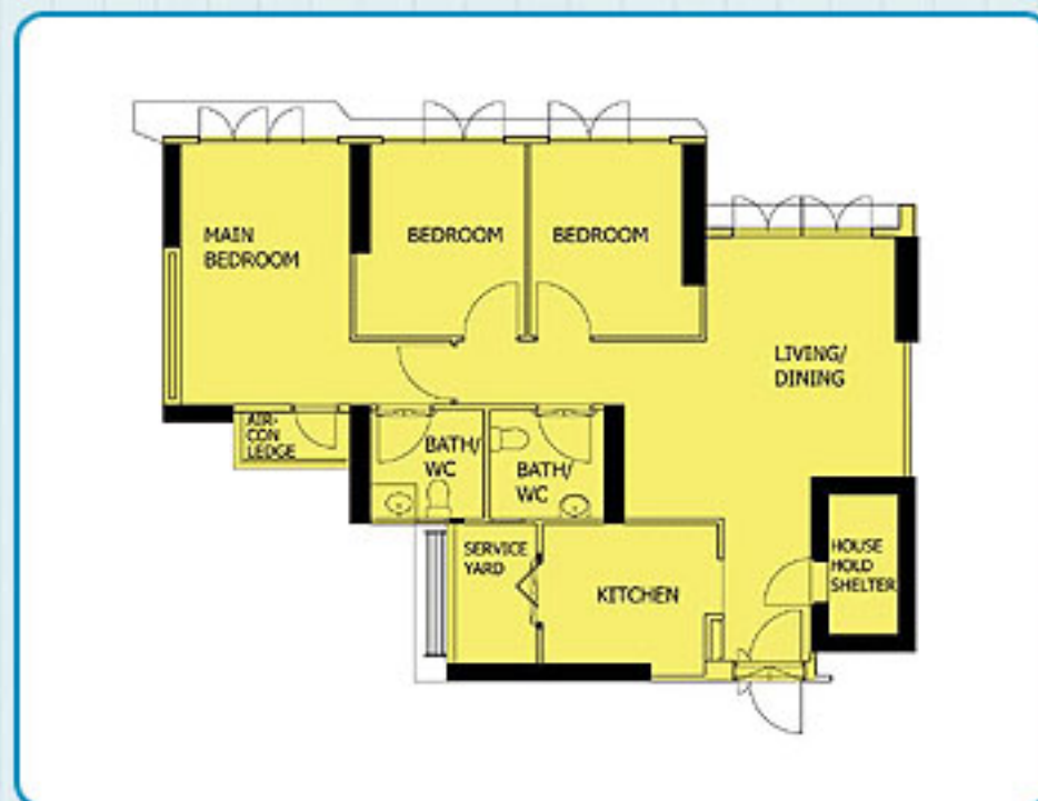
TYPICAL 4-ROOM FLOOR PLAN APPROX. FLOOR AREA 92 sqm (Inclusive of Internal Floor Area 90 sqm and Air-Con Ledge)
