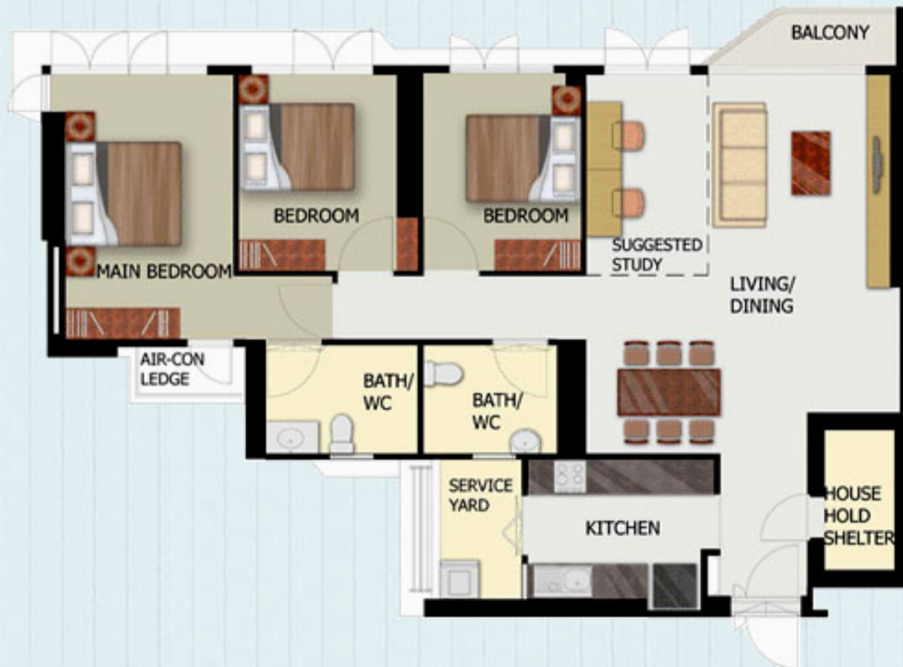
TYPICAL 5-ROOM FLOOR PLAN WITH BALCONY APPROX. FLOOR AREA 115 sqm (Inclusive of Internal Floor Area 113 sqm and Air-Con Ledge)
