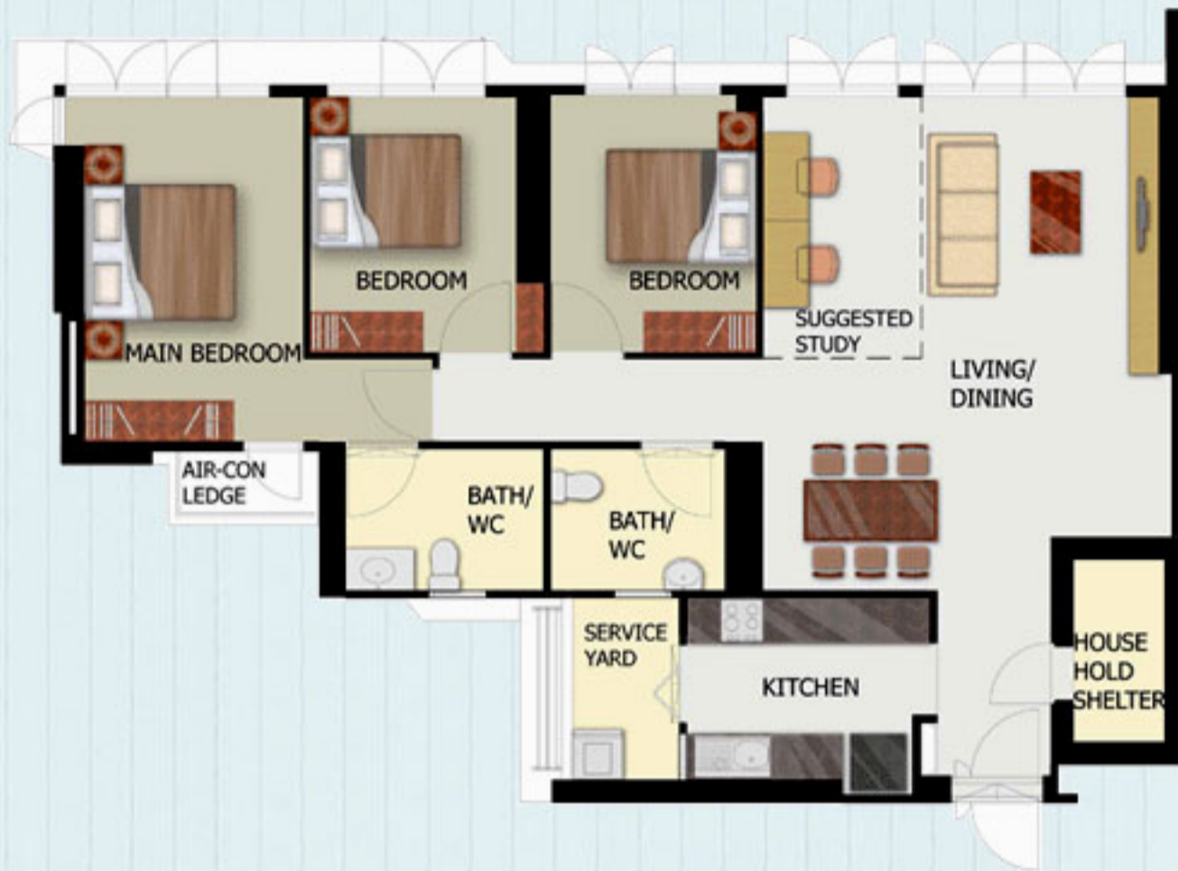
TYPICAL 5-ROOM FLOOR PLAN APPROX. FLOOR AREA 112 sqm (Inclusive of Internal Floor Area 110 sqm and Air-Con Ledge)
